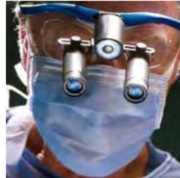
The K-LED head light produces a homogeneous light patch of up to 18000 lux. The 3W LED is mounted paraxially on the loupe bar and is powered by a lithium battery pack allowing 4 hours of continuous use.
